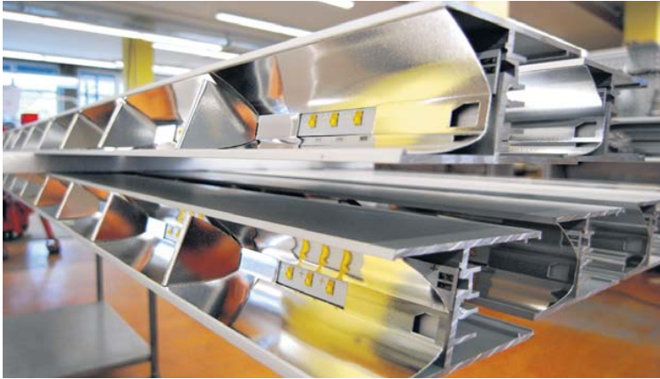
LED-Schienen in der Endmontage.
